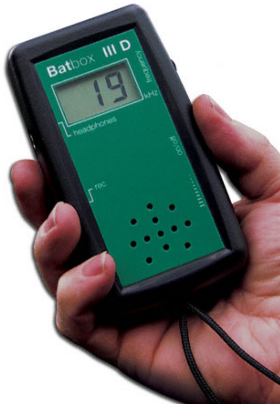
Batbox heterodyne bat detektor
