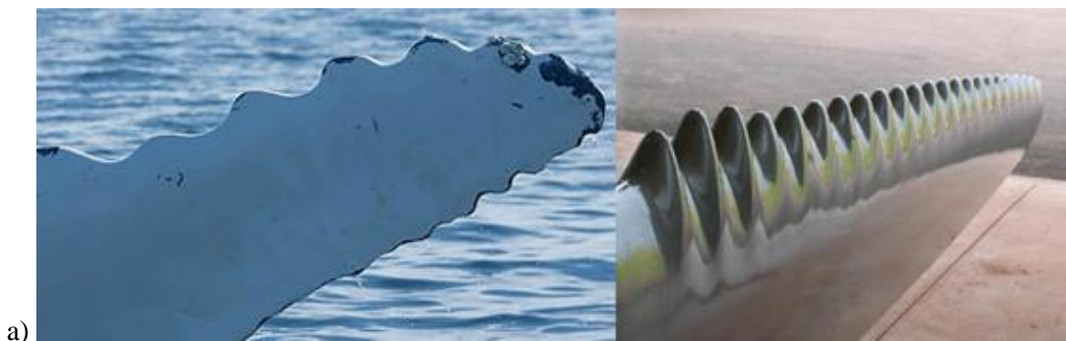
Figure 7. Humpback whale pectoral fin with tubercles and a prototype of a wind turbine blade [22]
